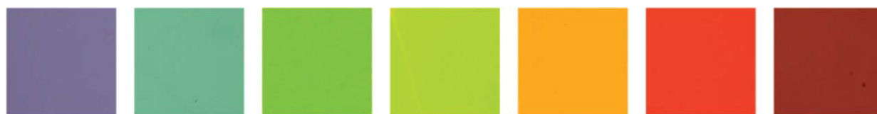
Fig. 7 Pictures of the 5 \mu\text{m} cell with 15 wt% 4a in E31 taken by a microscope in the crossed-polarized reflective mode from a dark state to the excited state under UV irradiation at 365 nm for different times: 6 s, 20 s, 30 s, 40 s, 50 s, 60 s and 70 s.
